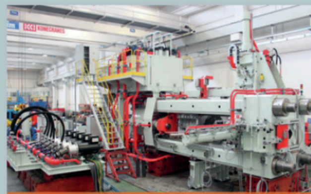
33 MN Front Loading Extrusion Press equipped with PE. Energy Saving System Pressa da 33 MN a caricamento frontale equipaggiata con PE. Energy Saving System
