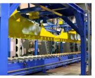
automatically from the die oven area assembly/storage area to the die oven zone for subsequent loading into the press. The same monorail will also be able to transfer dies automatically from the die storage area assembly/ storage area to the die oven zone.
