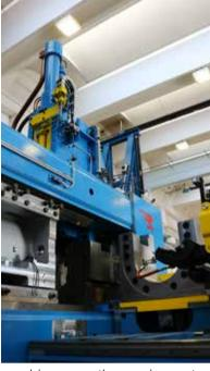
machine, as the main motor unit, the puller jaw rotation, jaw height adjust and IN/OUT of the iaws are foreseen by means of AC drives with frequency converter installed on board of the carriage.
