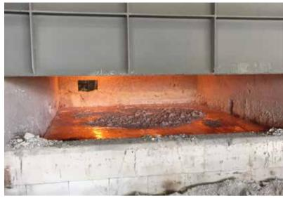
Without stirring the submerged scrap would take a very long time to melt down as it relies on conduction and convection heat transfer. Stirring the bath breaks this limitation and the heat transfer is greatly increased by convection effects.
