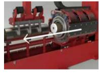
The oven moves on special guides with rollers and is actuated by a linear actuator electric provided with servomotor
