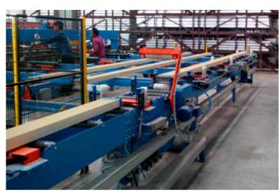
The wrapping line is equipped with a loading table that automatically feed the wrapper and the taping machine for the front end and back end of the packs. At unloading, a special bundle stacking machine, is able to form the packs with the insertion of a cardboard that protects the lower part during the forklift grip.
