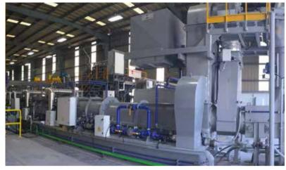
front loading press and a COIM log furnace with hot saw.
