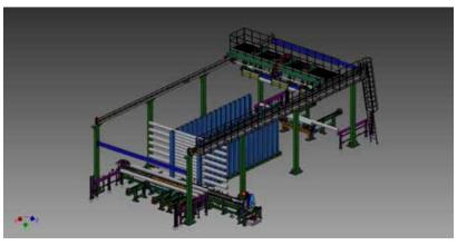
Not only billet heaters... COIM is highly specialized in strong, customized and fully automatic vertical storages for logs or pre-cut billets.
